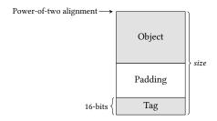
Fig. 5. PAMD's approach for inline metadata. "Object" is aligned to a power-of-two boundary and "padding" is inserted to ensure *size* is a power-of-two.
